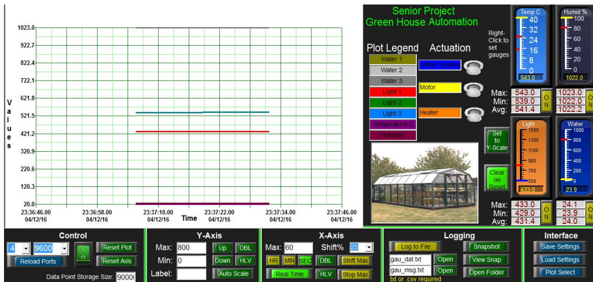
Fig. 9: The Control Panel for BU Greenhouse Project
