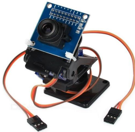
Fig. 7: A 2-Axis FPV Camera Cradle Head and OV7670 Camera Set sold by Next) seven.
