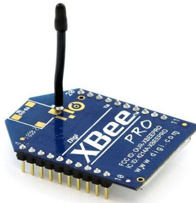
Fig. 2c: XBee Pro 60mW Wire Antenna - Series 1 (802.15.4), 250kbps max data rate,60mW output (18dBm), 1 mile (1600m) range, and a built-in antenna. Fully FCC certified.
