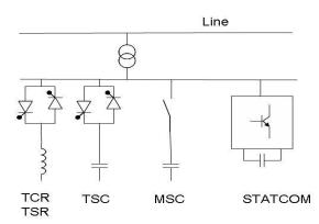
Fig 6: Examples of FACTS For Shunt Compensation
