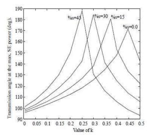
Fig 9. Variation in Transmission Angle at the Max SE power for diff. %S
