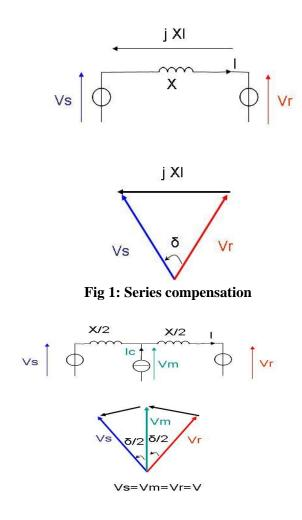
**Fig 2: Shunt Compensation**
