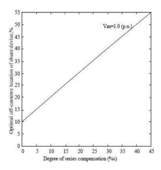
Fig 11: Variation in the Optimal Off-Center Location of Shunt FACTS Device against Degree of Compensation of Line (%S)
