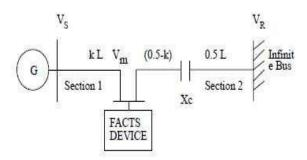
Fig 3. 2: Port, 4-Terminal Model of a Transmission Line
